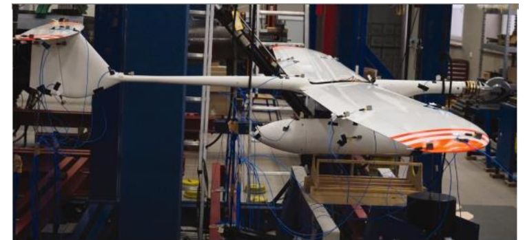
Ground vibration test (GVT) for full-scale UAVs
